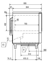
Drain Electrical inlet (power)
